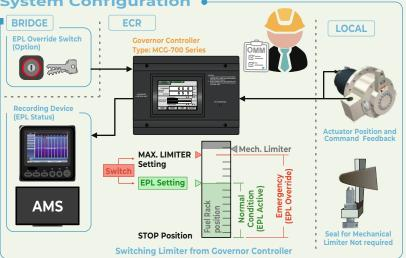
The EPL is one of the solution which complies with the MEPC technical guidelines for EEXI "GUIDELINES ON THE SHAFT / ENGINE POWER LIMITATION SYSTEM TO COMPLY WITH THE EEXI REQUIREMENTS AND USE OF A POWER RESERVE"
